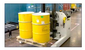
5. Blanks are cut from sheet metal and shipped to the Mint in drums.
