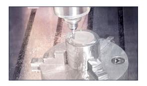
4. However the model is made, the design is then cut directly into steel using a computer-controlled engraving machine. This process takes up to 24 hours.
