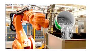
6. Titan (one of the Mint's robots) tips the blanks into a hopper and they travel along a conveyor belt to the coin presses.
