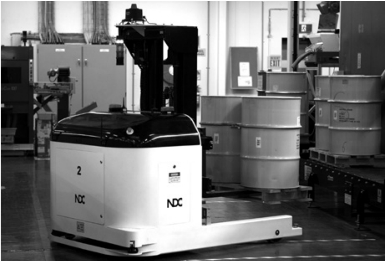
AGV transferring drums in the circulating coin production area.
